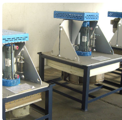
Before dispatch all hot gas circulating fans will be checked at the test bench for unbalance and power
